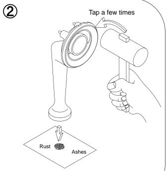
Tap the Burner Head a few times with a plastic or wooden hammer to remove the rust and ashes.
